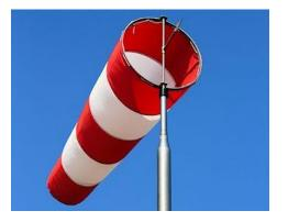
The white and orange blocks on a windsock indicate relative wind speeds. If just the first block is inflated but the rest is not, then the wind is approximately 3 knots. Each block represents an additional 3 knots. This windsock indicates a wind speed of at least 15 knots.
